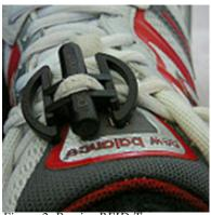
Figure 2: Passive RFID Tag – marathon race chip. Source: Yoppy used under <u>CC BY</u>
